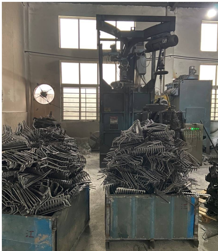
Shot Blasting - Material Handling
